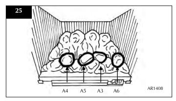
• Place the next four pebbles as identified resting between the flame baffle and the first row of pebbles as shown in Diagram 26
